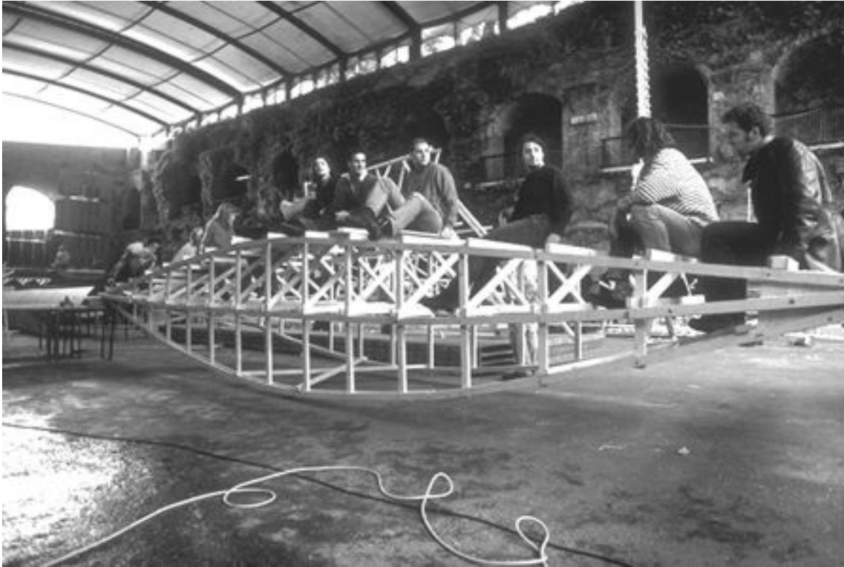
Fig. 3 Bridge made of roof battens, span: 8 metres (The truth about efficiency).
