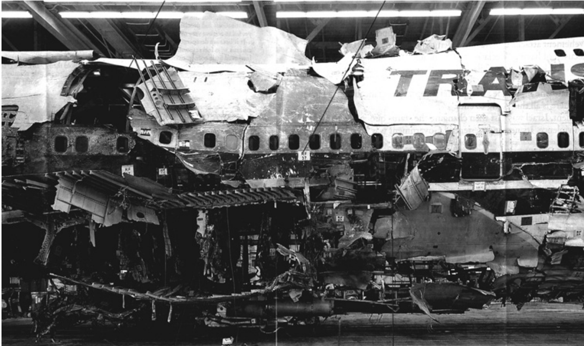
Fig. 6 Large photograph of TWA flight 800, reassembled in aircraft hanger in order to understand what happened to the airplane. Simulation to understand what happened vs. simulation to understand what is going to happen is the same [New York Times Magazine - 11 May 1997, pp. 38-39]
